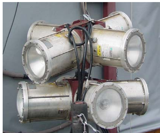
Figure 3. Underwater strobe lights (Flash Technologies, Inc.) used in effectiveness testing at Dworshak Dam.
