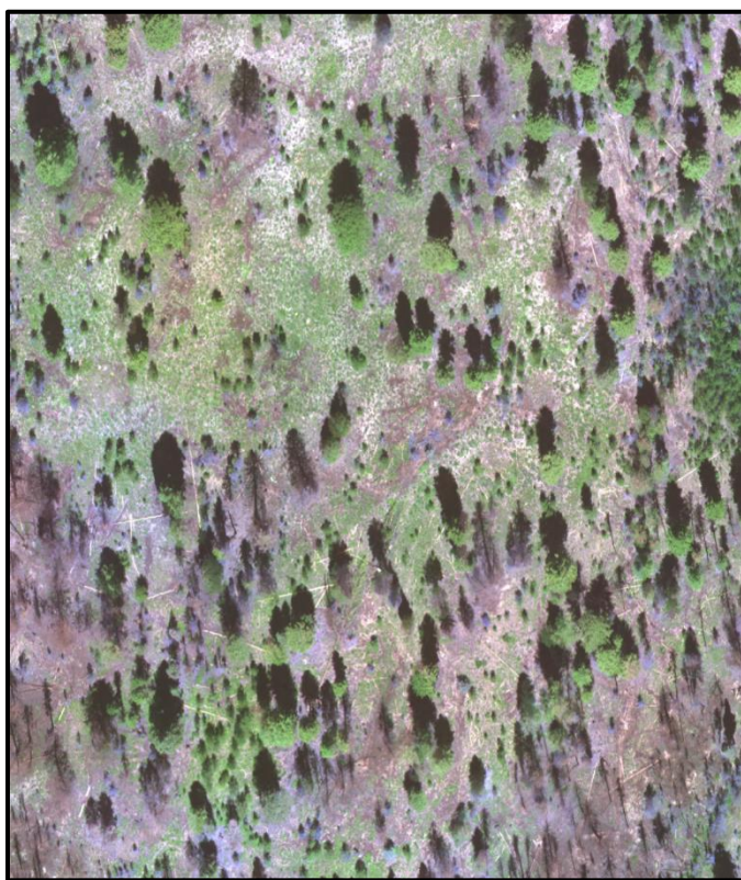
Figure 3. Small unmanned aerial system (sUAS) derived image mosaic of a female mule deer forage vegetation plot in the Whitehawk basin of Idaho. This image composite of several hundred individual sUAS images has a resolution of slightly larger than 7.4 cm.
